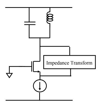
Feedback can be from drain to source or gate to source
