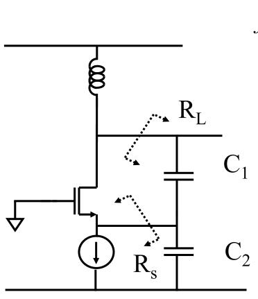
$$f_{o} = \frac{1}{2\pi\sqrt{L \cdot (\frac{C_{1} \cdot C_{2}}{C_{1} + C_{2}})}}$$
