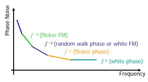
$$\mathcal{L}_{total}\{\Delta\omega\} = 10 \cdot \log \left[ rac{P_{sideband}(\omega_0 + \Delta\omega, 1Hz)}{P_{carrier}}
