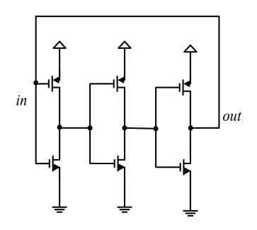
$$H(j\omega_0) = \left(\frac{-GmR_0}{1 + j\omega_0 R_0 C_0}\right)^N$$
